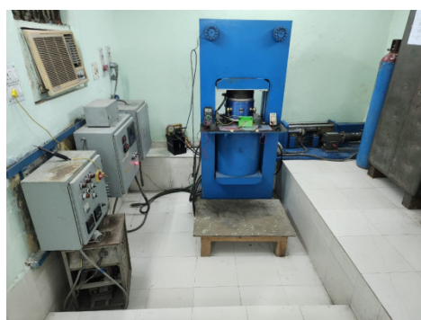
Walker-type Multi-Anvil High Pressure (50 GPa) and Temperature (2500°C) apparatus.
