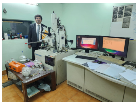
JEOL-JXA (Superprobe) Electron Microprobe for BSE-SEM and micron-size point analysis of natural and synthetic materials.
